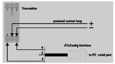
ATxRail-ATxConfig Adaptor wiring (loop powered). Terminal 5 is left opened.
